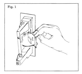
The magnet that is fitted to the mechanism, should be kept clean from foreign particles. The magnet can be cleaned by swinging the gate open. (as shown in Fig. 1). Remove metal filings from the magnet by guiding the point of a screwdriver along the edges of the magnet, such that the filings cling to the screwdriver.
