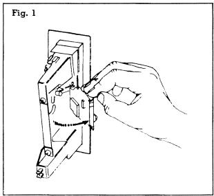
The magnet that is fitted to the mechanism, should be kept clean from foreign particles.
