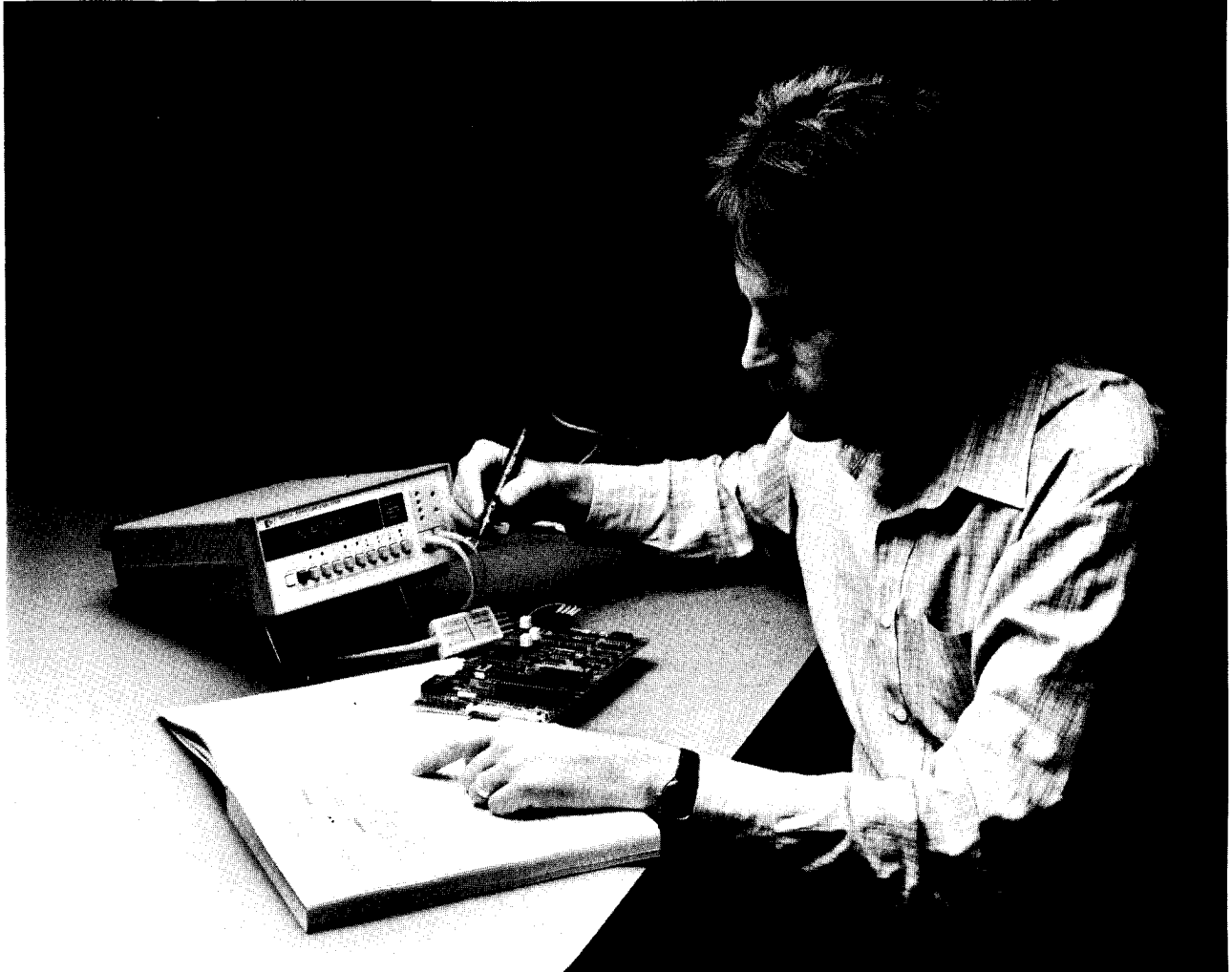
Figure 1. Composite signature saves time by reducing the amount of visual comparisons the troubleshooter must make to printed documentation. The HP 5006A Signature Analyzer is the first signature measurement instrument to offer this capability.
