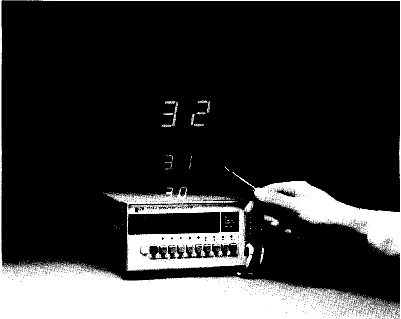
Figure 5. The operator can concentrate on probing without referring to the display using the signature memory in the HP 5006A. This makes misprobes and miscounts less likely. Time is saved when composite signature does not match because individual signatures do not need to be reprobed. The memory can be reviewed in the RECALL mode by pressing the probe switch and then compared to printed tables.
