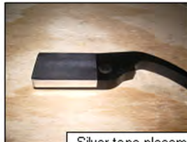
Silver tape placement (2W500) on black toggle (WACP0031)
