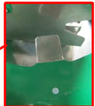
Silver tape placement (2W500) on black toggle (WACP0031)
